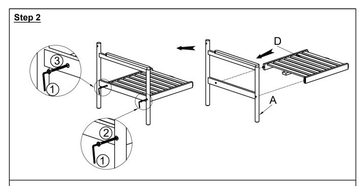
With assistance from your partner, attach Seat Panel (D) to Left Leg Panel (A) by using 2 Screws (2)+(3) and Allen Wrench (1) as shown above.
