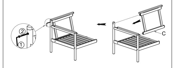
Attach Backrest Panel (C ) to Left Leg Panel (A) by using Screw (2) and Allen Wrench (1).
