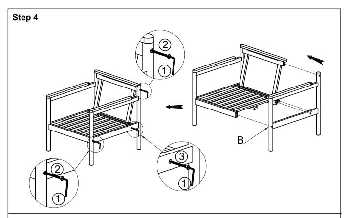
Attach Right Leg Panel (B) to Backrest Panel (C) and Seat Panel (D) by using Screws (2), Screw (3) and Allen Wrench (1).
