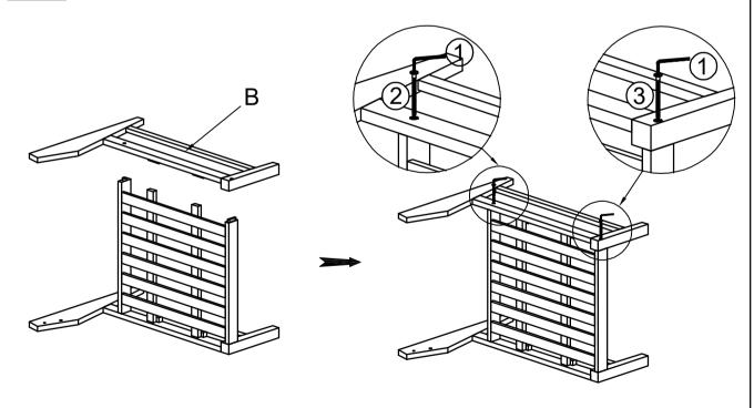
Flip the Chair to the side as shown. Attach Right Leg Panel (B) to Seat Panel (C) by using 2 Screws (2)+(3) with Allen Wrench (1) to secure.
