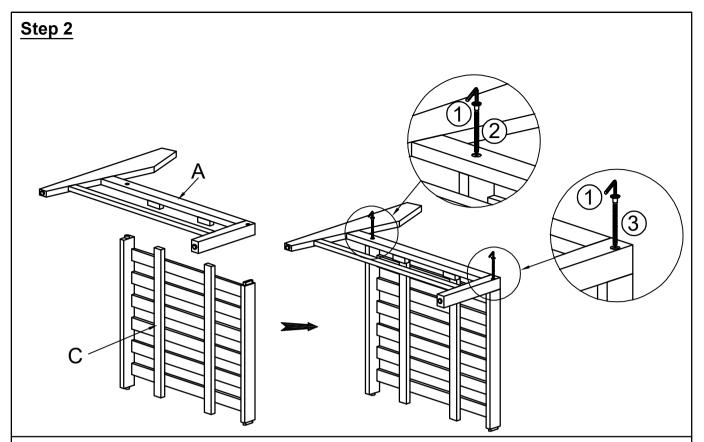
Place Seat Panel (C) as above picture. Attach Left Leg Panel (A) to Seat Panel (C) by using 2 Screws (2) +(3) with Allen Wrench to secure.
