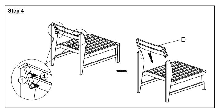
Attach Backrest Panel (D) to Left Leg Panel (A) and Right Leg Panel (B) by using 4 Bolts (4) with Allen Wrench to secure.
