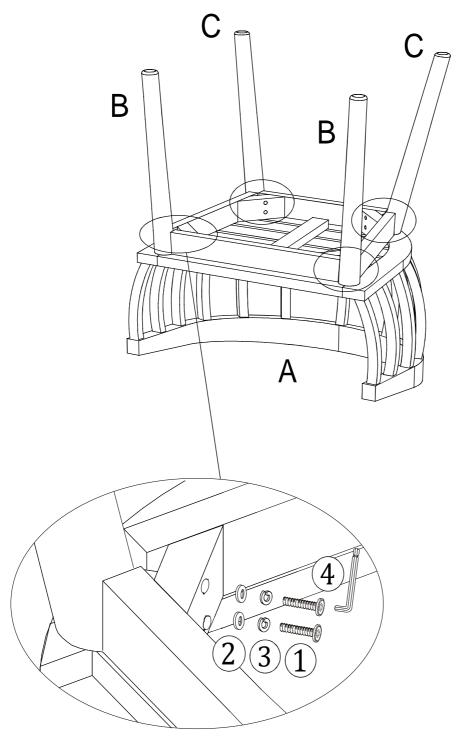
With the help of your adult partner, place the Seat Panel (A) with its underside skywards onto a clean, soft surface to avoid any scratch or damage to the product.
