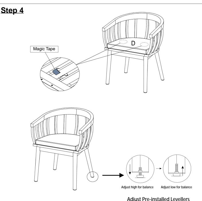
Adjust Pre-installed Levellers high for balance
