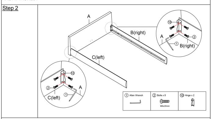
Attach the Side rail B (right) and Side rail C (left) to the Head board A by using Bolts ② and Hinge ⑩ with Allen Wrench ①.
