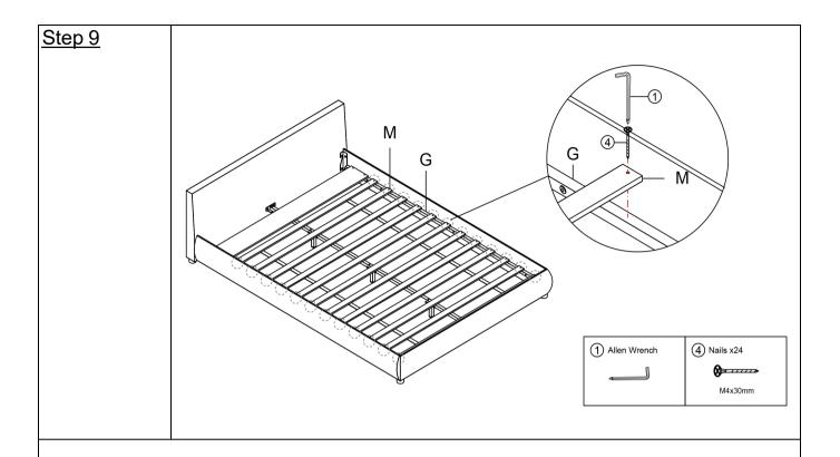
Attach the Slat M to the Side rails support bar G by using Nails ④ with Allen Wrench ①.
