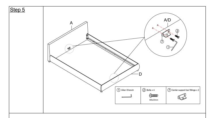
Attach the Center support bar fittings ⑦ to the Head board A and Foot board D by using Bolts ② by with Allen Wrench ①.
