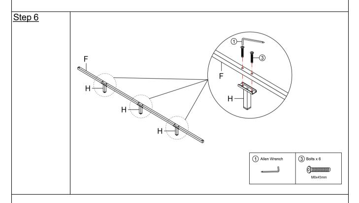
Attach the Middle support leg H to the Center support bar F by using Bolts ③ by with Allen Wrench ①.
