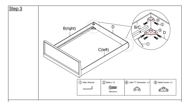
Attach the Foot board D to the Side rail B (right) and Side rail C (left) by using Bolts ②,Metal Corner ⑨ and Little "7" Connector ⑧ with Allen Wrench ①.
