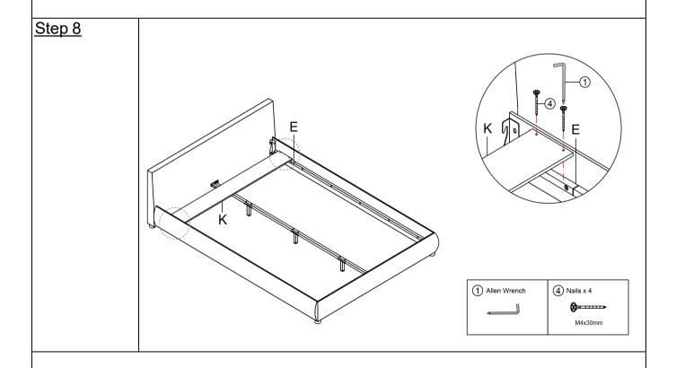
Attach the Cross board K to the Side rails support bar E by using Nails ④ with Allen Wrench ①.
