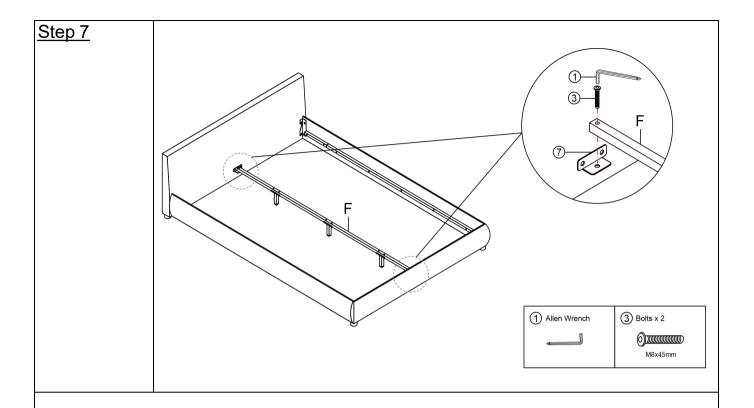
Attach the Center support bar F to the Center support bar fittings ⑦ by using Bolts ③ with Allen Wrench ①.
