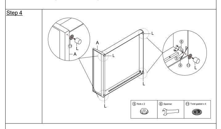
Attach the Bed legs L and Twist gasket ① to the Head board A.
