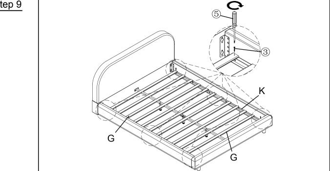
Attach Slats (G) to Side rails support bar (K) by using Screws (③) with Screwdriver (5).
