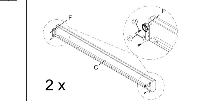
Attach V-Bracket (F) to 2 x Side Rail (C) by using Bolts (2) with L-Allen Key (4).
