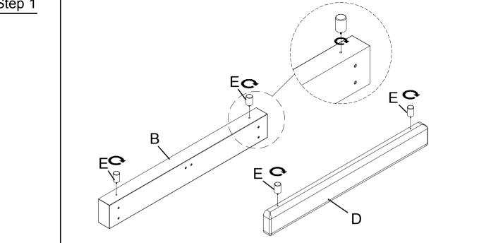
Attach Leg Bed (E) to Headboard (B) and Footboard (D).
