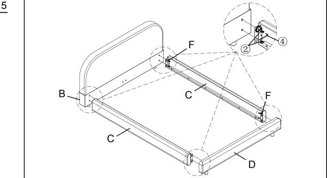
Attach V-Bracket (F) and Side Rail (C) to Under Headboard (B) by using Bolts (2) with L-Allen Key (4),
