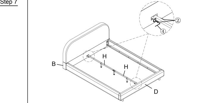
Attach Center Rail (H) to Under Headboard (B) and Footboard (D) by using Bolts (②) with L-Allen Key (④).
