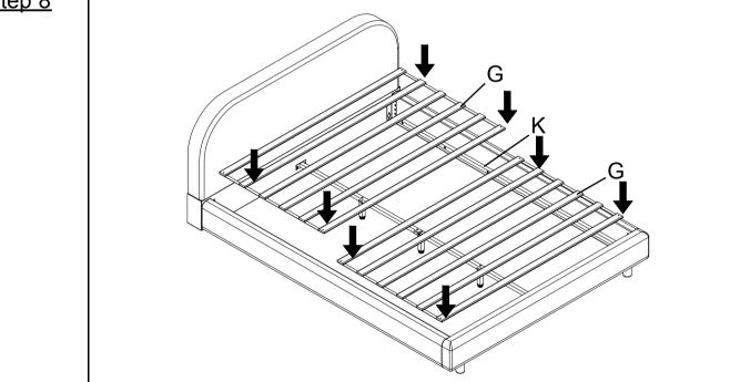
Attach Slats (G) to Side rails support bar (K).
