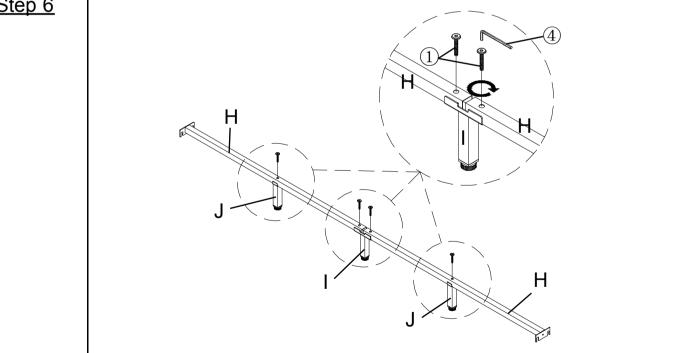
Attach Center Rail (H) to Support Leg (J) by using Bolts (1) with L-Allen Key (4), Attach Center Rail (H) to Center Leg (I) by using Bolts (1) with L-Allen Key(4).
