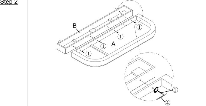
Attach Headboard (A) to Under Headboard (B) by using Bolts (1) with L-Allen key (4).
