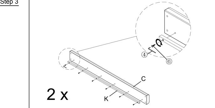
Attach Side rails support bar (K) to 2 x Side Rail (C) by using Bolts (6) with L-Allen Key (4).
