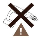
The use of power tools to assemble this product could lead to damage, making it unsafe
