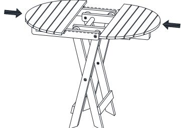
Push the 2 wings back so that the locating pin and the waiting hole match as shown.
