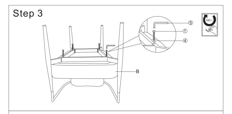
Attach the Seat Cushion (B) to the frame using Washer (4),Bolt (1) with Allen Wrench (5) as pictured above. Fully tighten the Bolts.
