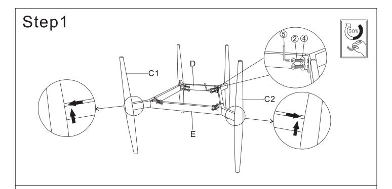
Attach the Back Connection Rod (D) and Front Connection Rod (E) to L leg(C1) and R leg(C2) using the Washer (4),Bolt (2) with Allen Wrench (5) as pictured above.
