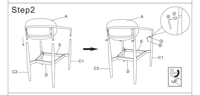
Attach the assembled Back (A) to frame with Leg using Threaded Rod (3) with Allen Wrench (6) as pictured above. Do not fully tighten the Bolts.
