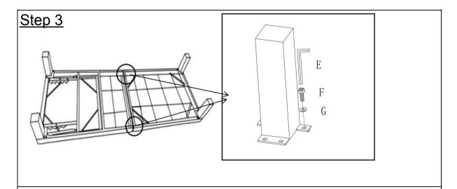
Attach Middle Legs(D) to the Seat Panel(A) using Bolts(F) with Allen Key(E).
