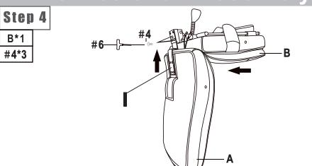
As shown in the figure, insert the other end of the connecting piece 'H' into the interface behind the cushion and fix it with 3 screws numbered '#4'.
