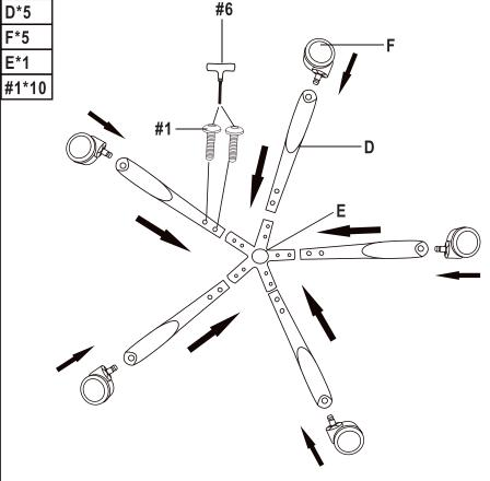
First, we need to prepare the connector (**E**), 5\* metal feet (**D**), 5\* universal wheels (**F**), 10\*16mm screws (# **1**) and a wrench (# **6**). Then, according to the figure, insert the 5\* metal feet into the connector, align the screw holes, install the screws and tighten them. Finally, a universal wheel is installed on the tail of each metal foot.
