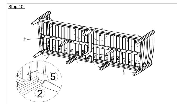
With the help of your adult partner, place the assembled parts in Step 9 to the assembled part in Step 8 and then secure by using Screws (2) and Allen Wrench (5) as shown above.
