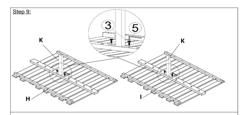
With the help of your adult partner, place the Left Seat Panel (H) facing down, then attach the Support Leg (K) to the Left Seat Panel (H) and secure by using Screws (③) and Allen Wrench (⑤).
