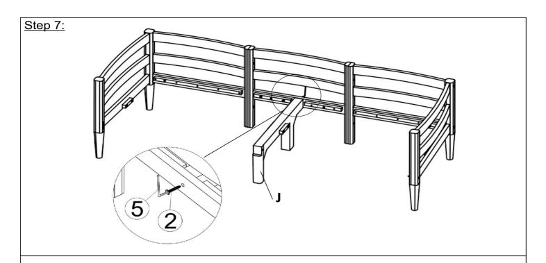
With the help of your adult partner, attach the Front Middle Leg (J) to the assembled part in Step 6 and then secure the Front Middle Leg (J) to the Middle Leg Panel (F) by using Screws (②) and Allen Wrench (⑤) as shown above.
