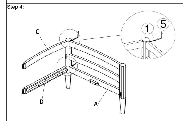
With the help of your adult partner, put the tenons of the Back Slat (C) and Back Support Bar (D) to the mortises of Right Leg Panel (A) and then secure by using Screws ( $\mathfrak{D}$ ) and Allen Wrench ( $\mathfrak{D}$ ) as shown above.
