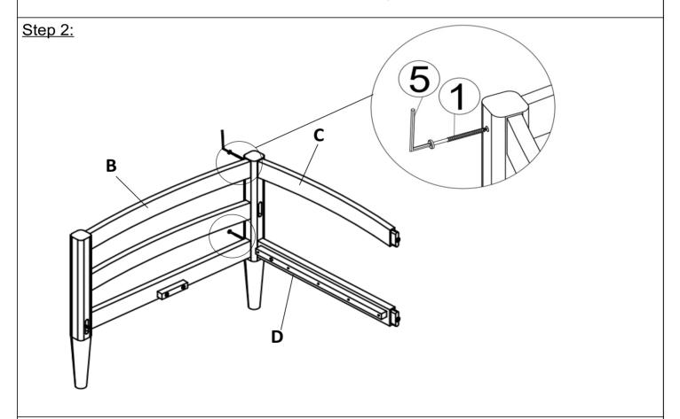
With the help of your adult partner, put the tenons of the Back Slat (C) and Back Support Bar (D) to the mortises of Left Leg Panel (B) and then secure by using Screws (1) and Allen Wrench (5) as shown above.
