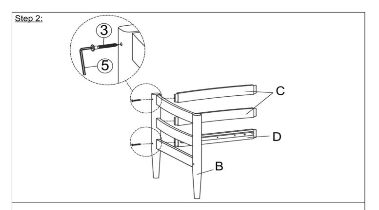
With the help of your adult partner, put the tenons of Back Slats (C) and Back Support Bar (D) to the mortises of Left Leg Panel (B) and then secure by using Screws ( $\Im$ ) and Allen Wrench ( $\Im$ ) as shown above.
