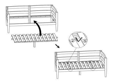
With the help of your adult partner, place the assembled part in Step 7 to the assembled part in Step 6 and then secure the Seat Panel (I) to the Back Support Bar (D) and Front Support Bar (E) by using Screws Screws (②) and Allen Wrench (⑤) as shown above. **Do not fully tighten the Screws.**
