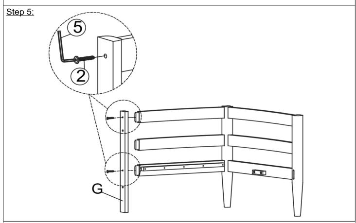
With the help of your adult partner, put the mortises of Right Middle Leg (G) to the tenons of Back Slats (C) and Back Support Bar (D) of the assembled part in Step 4 and then secure by using Screws (2) and Allen Wrench (5) as shown above.
