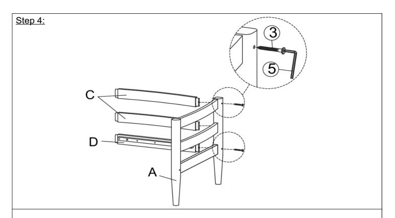
With the help of your adult partner, put the tenons of the remaining Back Slats (C) and Back Support Bar (D) to the mortises of Right Leg Panel (A) and then secure by using Screws (3) and Allen Wrench (5) as shown above.
