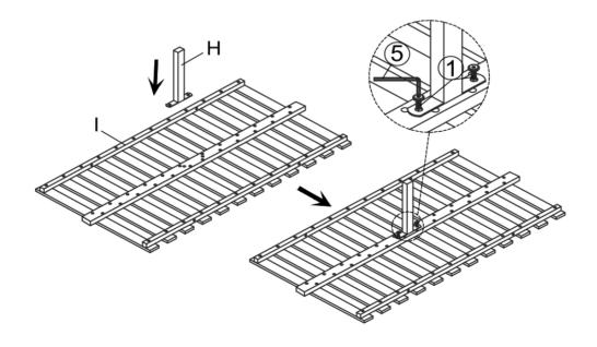
With the help of your adult partner, place the Seat Panel (I) facing down and then attach the Support Leg (H) to the Seat Panel (I) by using Screws (1) and Allen Wrench (5) as shown above.
