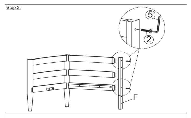
With the help of your adult partner, put the mortises of Left Middle Leg (F) to the tenons of Back Slats (C) and Back Support Bar (D) of the assembled part in Step 2 and then secure by using Screws (2) and Allen Wrench (5) as shown above.
