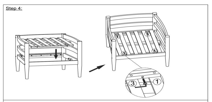
Place the Seat Panel (F) to the assembled part in Step 3 and then secure the Seat Panel (F) to the Back Support Bar (D) and Front Support Bar (E) by using Screws (1) and Allen Wrench (3) as shown above.
