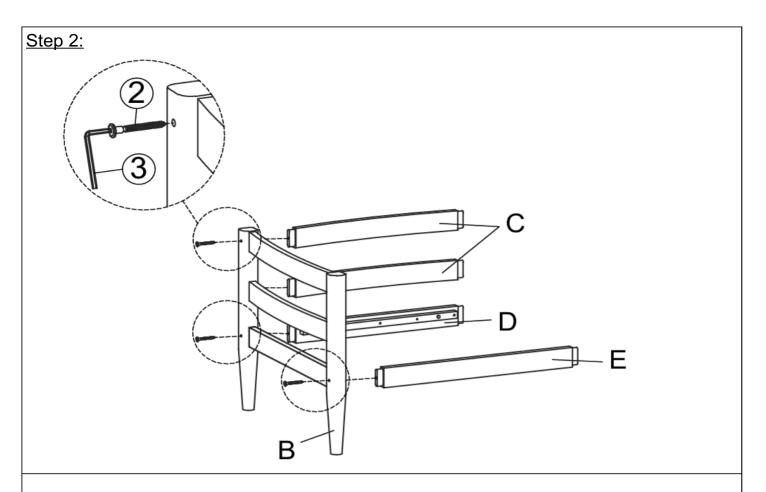
With the help of your adult partner, put the tenons of Back Slats (C), Back Support Bar (D) and Front Support Bar (E) to the mortises of Left Leg Panel (B) and then secure by using Screws (②) and Allen Wrench (③) as shown above.
