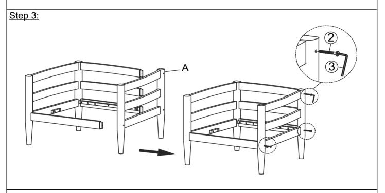
With the help of your adult partner, put the mortises of Right Leg Panel (A) to the tenons of Back Slats (C), Back Support Bar (D) and Front Support Bar (E) of assembled part in Step 2 and then secure by using Screws (2) and Allen Wrench (3) as shown above. **Do not fully tighten the Screws.**
