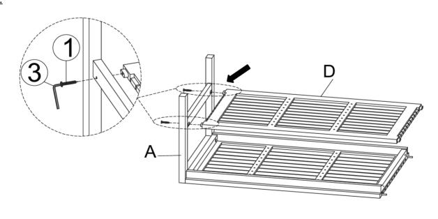
With the help of your adult partner, attach the Table Shelf (D) to the assembled part in Step 2 and then secure the Table Shelf (D) to the Left Leg Panel (A) by using Screws ( $\mathfrak{I}$ ) and Allen Wrench ( $\mathfrak{I}$ ) as shown above.
