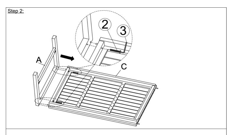
With the help of your adult partner, place the Table Top (C) with its underside skywards onto a clean, soft surface to avoid any scratch or damage to the product.
