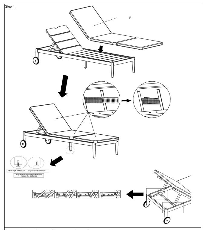
Inspect it and make sure all parts are adequately connected.
