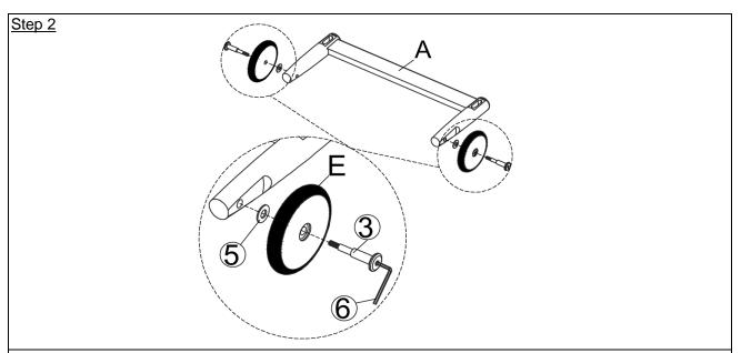
With the help of your adult partner, attach the Wheel (E) to the Back Leg Panel (A) by using Wheel Hub (3), Flat Washer (5) and Allen Wrench (6) as shown above.
