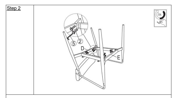
Attach the Connection Rod (D) and (E) to assembled Leg Frame using the Bolt (②) with Allen Wrench (⑤) as shown above.
