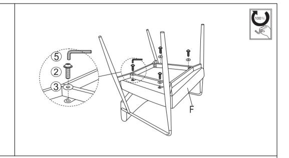
Attach the Seat Cushion (F) to assmbled frame using the Washer (③), Bolt (②) with Allen Wrench (⑤) as shown above.
