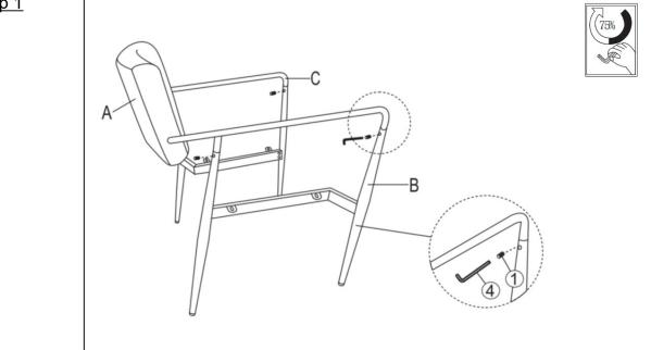
Attach the Chair Back(A) to the Left Leg (B) and Right Leg (C) ,using the bolt(1) with Allen Wrench (4) as shown above.
