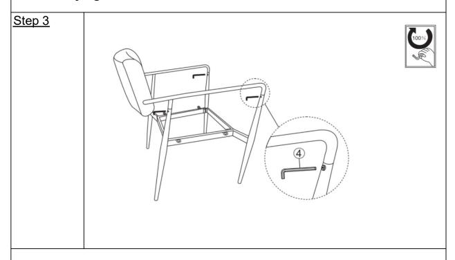
Stand the Chair up and fully tighten the Bolts.
