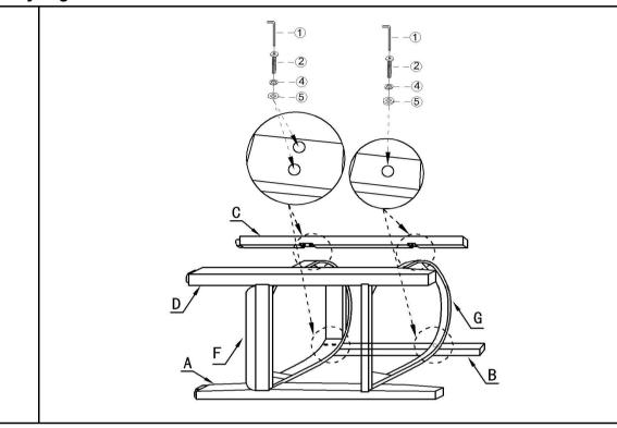
Insert the Left Hind Legs (B) and Right Hind Legs (C) onto the Seat Cushion (F) and Bottom Frame (G), use the Allen Wrench (F), Short Bolts (2), Spring Washer (4) and Flat Washer (5), as shown in the picture above.
