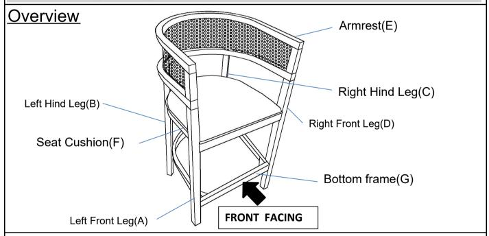
This Barstool has multiple parts and may require up to some 30 minutes to assemble. To give you an overview of the Barstool parts, the above picture is to help you put the various parts into perspective. Please read through the instructions below to familiarise yourself with the parts and steps before assembly.
