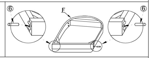
Install the Wooden Tenons(⑥) into the sides of the Seat cushion(F) as pictured above.
