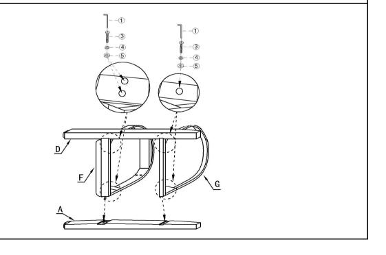
Plass the Left Front Leg (A) and Right Front Leg (D) to the Seat Cushion (F) and Bottom Frame (G), and then secure it with Allen Wrench (①), long Bolts (③), Spring Washer (④) and Flat Washer (⑤), as shown in the picture above.
