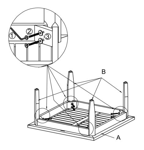
Attach Leg (B) to Top table (A) by using 8 Bolts (②), 8 Spring Washers (③) with Allen Wrench (①) as picture shown above.
