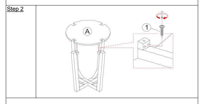
Attach Table top (A) on the Leg frame of Step 1 by using Wood screw (1) with Assembly Tools Required (Not Included) (2).
