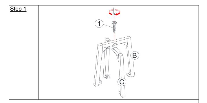
Attach Leg frame (B) on the Upper Leg frame (C) by using Wood screw (1) with Assembly Tools Required (Not Included) (2).
