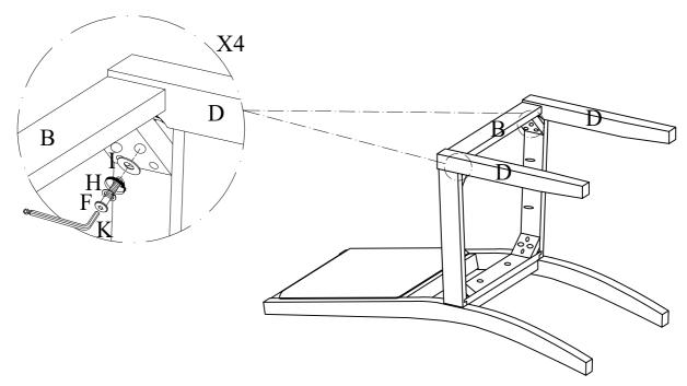
Take the Allen Wrench, and turn the bolts until the legs are secured. DO NOT TIGHTEN COMPLETELY.
