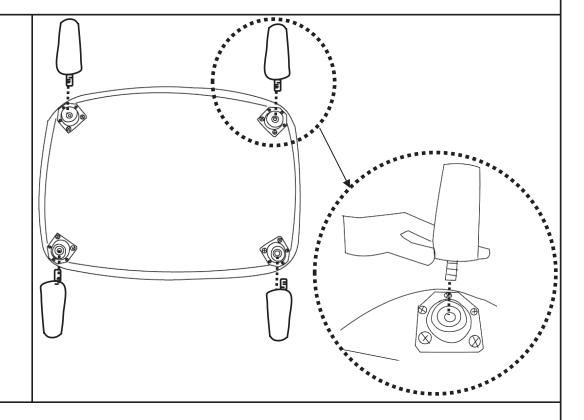
Screw the Wooden Leg(C) to the Frame(A) and gently tighten the legs.
