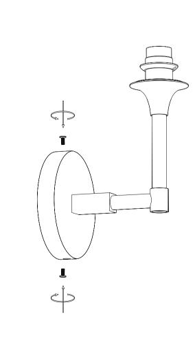
The main body of the light frame is locked on the hanging plate
