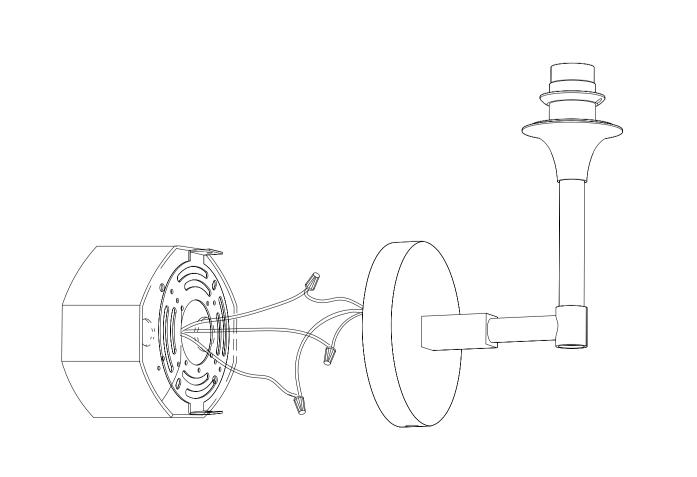
$\widehat{2}$  Connect the main power cable to the main lamp wire.
