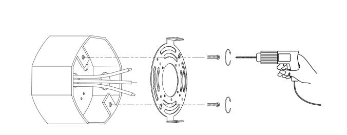
$\bigcirc$  Install the mounting plate on the wall.
