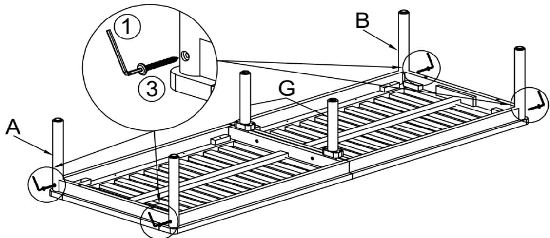
Keep place as pictured, attach Left Leg Panel (A) to Left Seat Panel (C) by using 2 Screws ③ with Allen Wrench (①).
