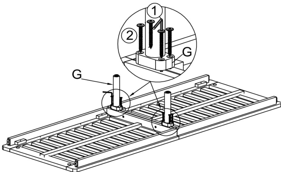
Attach 2 Middle Leg (G) to Left Seat Panel (C) and Right Seat Panel (D) as pictured by using 8 Screws (②) with Allen Wrench (①) to secure.
