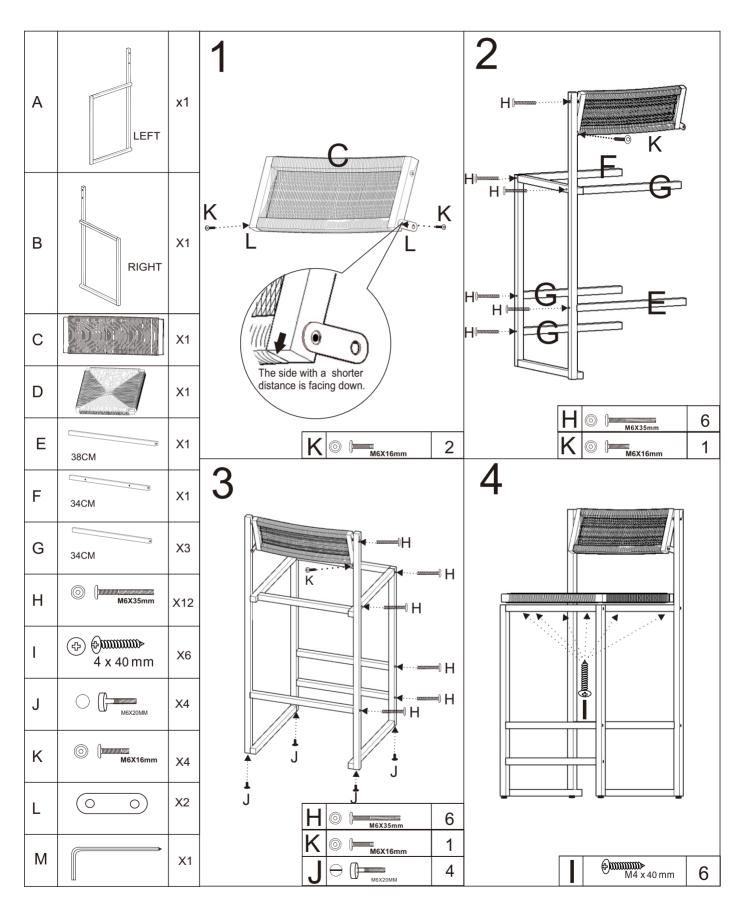
NOTE: There are no screw holes in seat D, seat D is made by wooden frame, please pass through the holes in metal frame with self-tapping screws (part I), then secure seat D by tightening self-tapping screws (part I).
