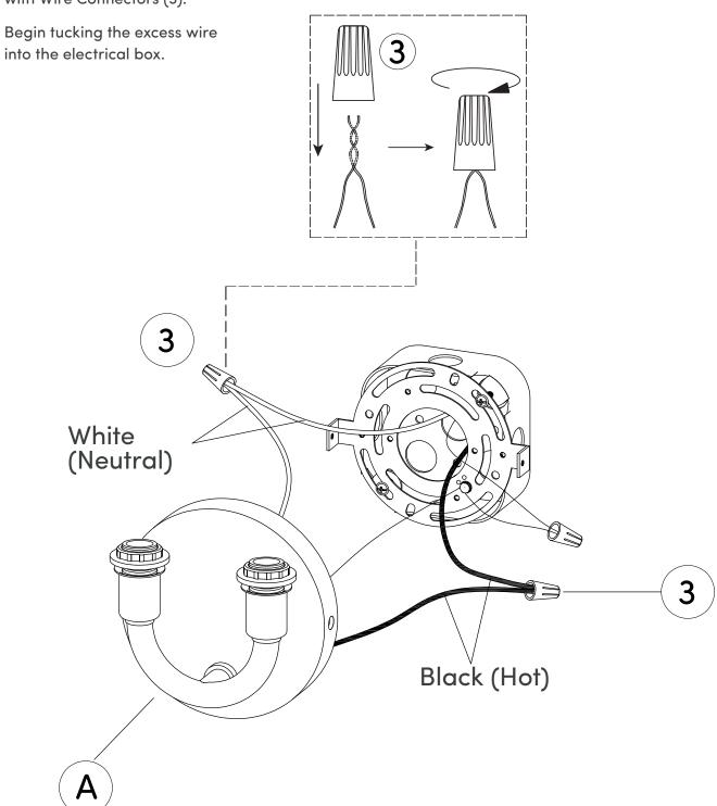
Using the Fixture Mounting Screws (4), mount the Fixture Assembly (A) to the Mounting Bracket (1).
