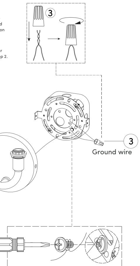
Join matching colored wires with Wire Connectors (3).
