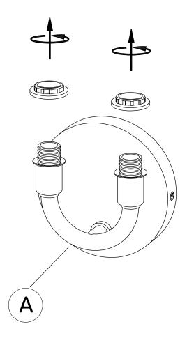
Secure the Shade (B) by twisting the shade collars back into place, sandwiching the shade between the shade collars and the Fixture Assembly (A).
