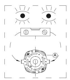
Ground Wire from the Fixture Assembly (A) is to be wrapped around the grounding screw on the Mounting Bracket.
