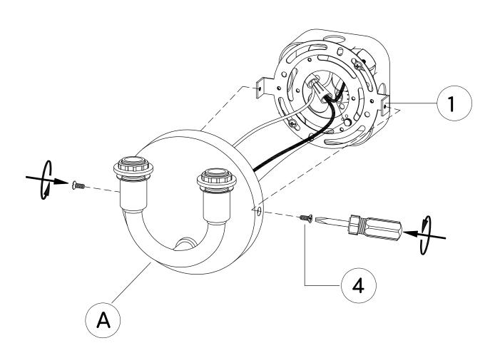
Remove the shade collars from the Fixture Assembly (A) by unscrewing them.
