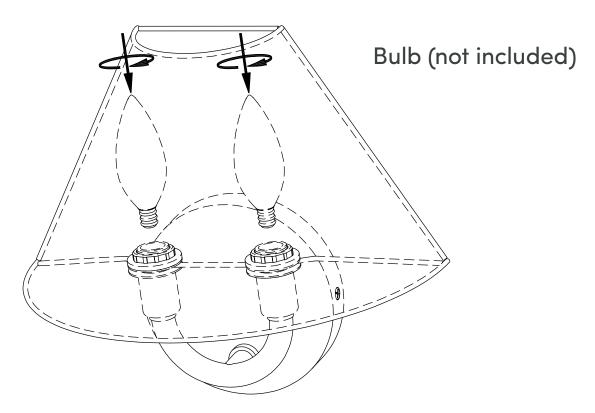
We recommend using 2 Type B10 or B11 light bulb. 120V 60Hz AC only.
