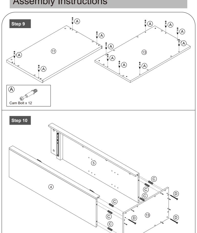
(C) Shininininin (D) 4\*35mm Screw x 4 8\*30mm Dowel x 6
