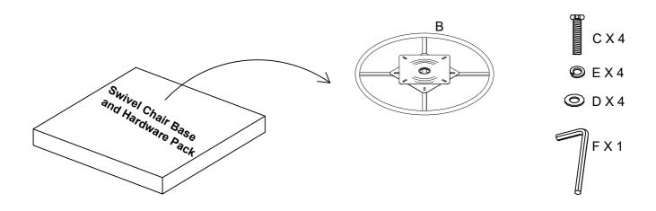
Turn the Chair (A) upside down and place it on a protective carpet. Attach the Swivel Chair Base (B) to the Chair (A) using Bolt (C), Spring Washer (E) and Flat Washer (D) with the Allen Wrench (F).
