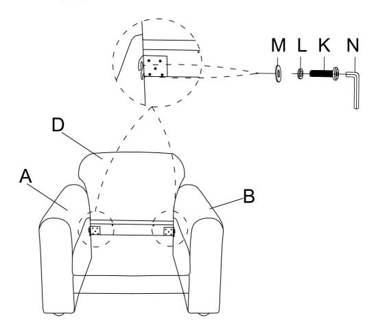
Flip the Chair to the bottom. Attach Seat Cushion Frame (E) to Back Rest (D) by L Bracket (I) using Bolt (K), Spring Washer (L) and Flat Washer (M) with Allen Key (N).
