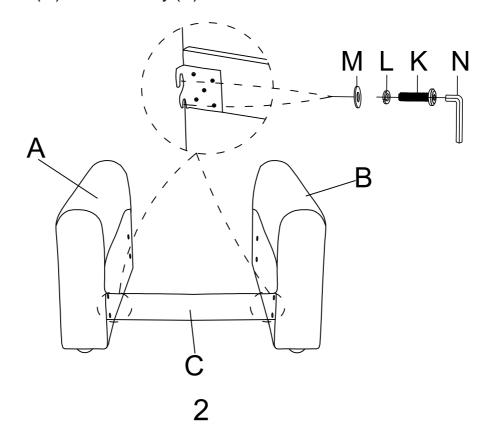
Attach Back Rest (D) to LSF & RSF Arm (A & B) using Bolt (K), Spring Washer (L) and Flat Washer (M) with Allen Key (N).
