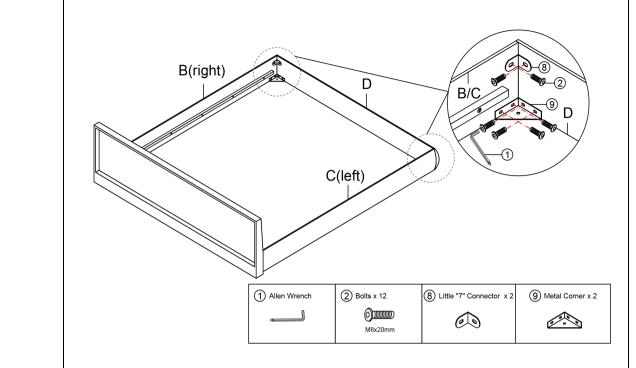
Attach the Foot board D to the Side rail B (right) and Side rail C (left) with Bolts ②, Metal Corner ⑨ and Little "7" Connector ⑧ by using Allen Wrench ①.
