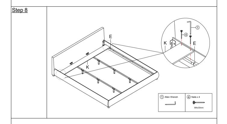
Attach the Cross board K to the Side rails support bar E with Nails ④ by using Allen Wrench ①.
