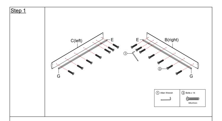
Attach the Side rails support bar E and Side rails support bar G to the Side rail B (right) and Side rail C (left) with Bolts ③ by using Allen Wrench ①.
