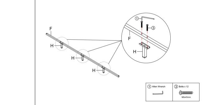
Attach the Middle support leg H to the Center support bar F with Bolts ③ by using Allen Wrench ①.
