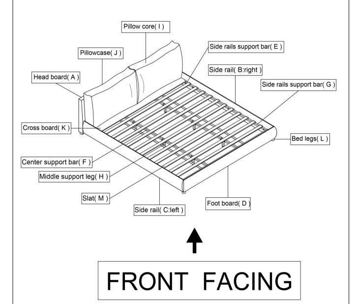
This Bed have multiple parts and may require up to 60 minutes to assemble. To give you an overview of the Bed parts, the above picture is to help you put the various parts into perspective. Please read through the instructions below to familiarise yourself with the parts and steps before assembly.
