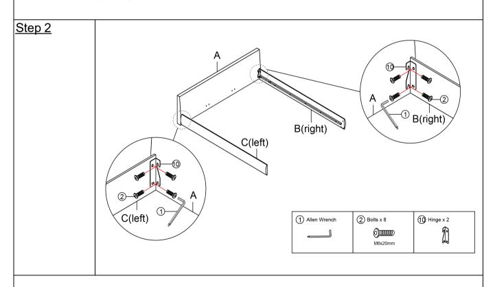
Attach the Side rail B (right) and Side rail C (left) to the Head board A with Bolts ② and Hinge ⑩ by using Allen Wrench ①.
