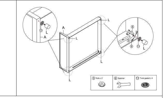
Attach the Bed legs L and Twist gasket ① to the Head board A.
