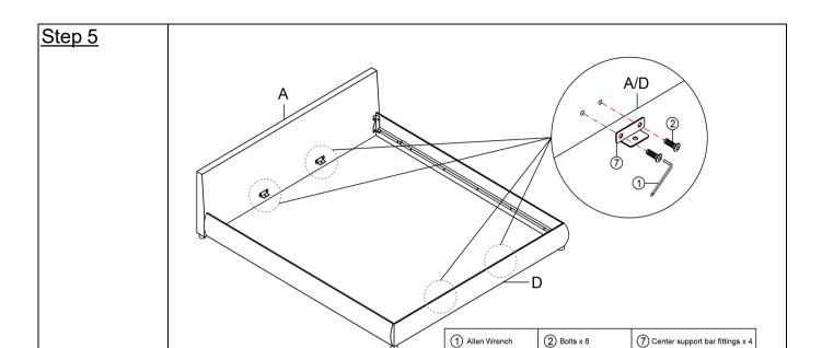
Attach the Center support bar fittings ⑦ to the Head board A and Foot board D with Bolts ② by using Allen Wrench ①.
