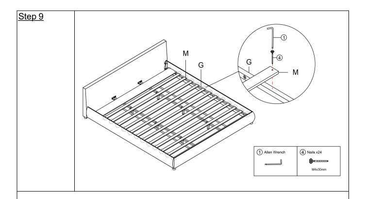
Attach the Slat M to the Side rails support bar G with Nails ④ by using Allen Wrench ①.
