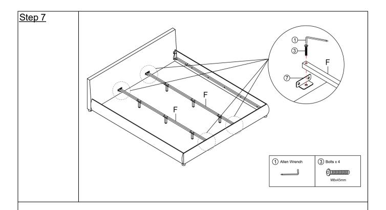
Attach the Center support bar F to the Center support bar fittings ⑦ with Bolts ③ by using Allen Wrench ①.
