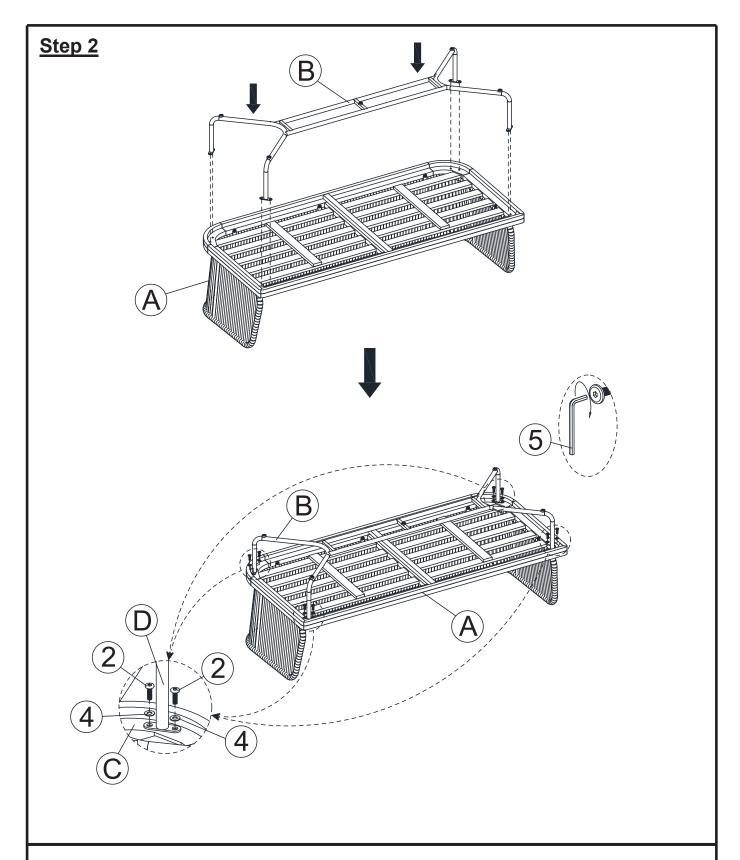
With assistance from your adult partner, place the seat frame (A) facedown onto a clean, non marring surface, then attach the Leg Frame (B) to the Seat Frame (A) using the Bolts (2), Washers (4) and the Allen Wrench (5).
