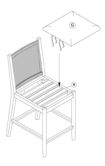
Secure the seat cushion straps by attach the Velcro together as shown in the image below.
