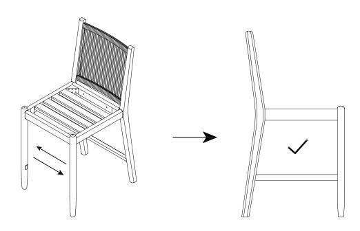
Carefully flip the stool over on a flat surface and make sure the legs are touching the ground evenly before tightening everything to 100%.
