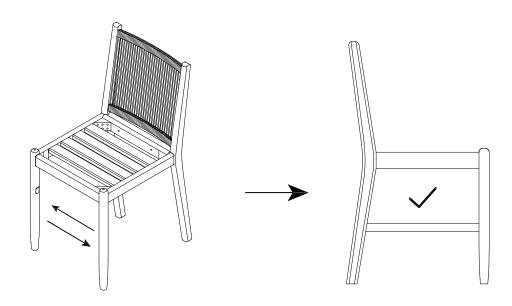
Carefully flip the stool over on a flat surface and make sure the legs are touching the ground evenly before tightening everything to 100%.
