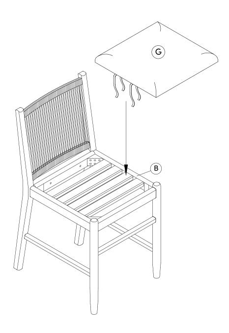
Secure the seat cushion straps by attach the Velcro together as shown in the image below.
