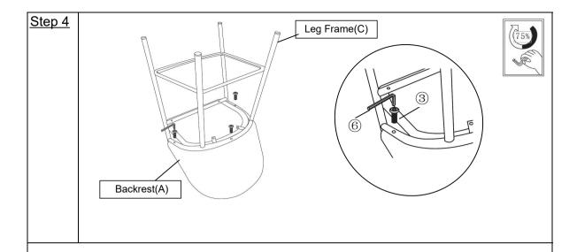
Attach the Chair Back(A) to assembled Leg Frame using the Bolt(M6x60mm)(③) with Allen Wrench(⑥) as pictured above.
