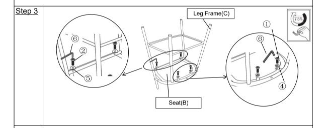
Attach the Foot Panel(D) to the Leg Frame(B) using Bolt(M6x40mm(2),Wash(5), Bolt(M6x20mm(1),Flat Washer(4) with Allen Wrench(6) as pictured above.
