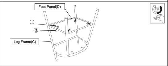
Attach the Foot Panel(D) to the Leg Frame(B) using Bolt(M6x20mm)(1) with Allen Wrench(6) as pictured above.
