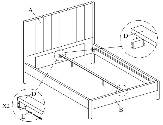
Attention: Please ensure that CSK Screw (L) is attached as shown to avoid the base from collapsing.
