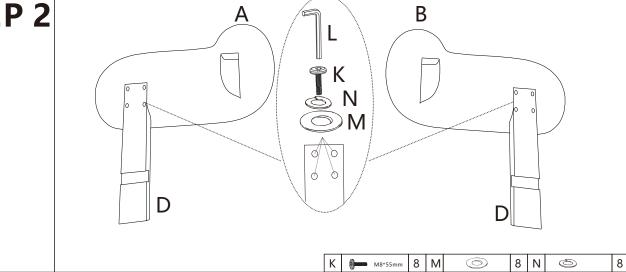
Assemble the leg(D) to the armrest(A and B) **Do not fully tighten the screws.**
