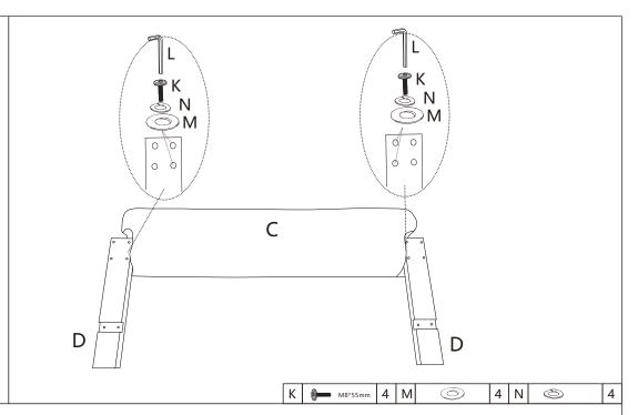
Assemble the leg(D) to the backrest(C). **Do not fully tighten the screws.**
