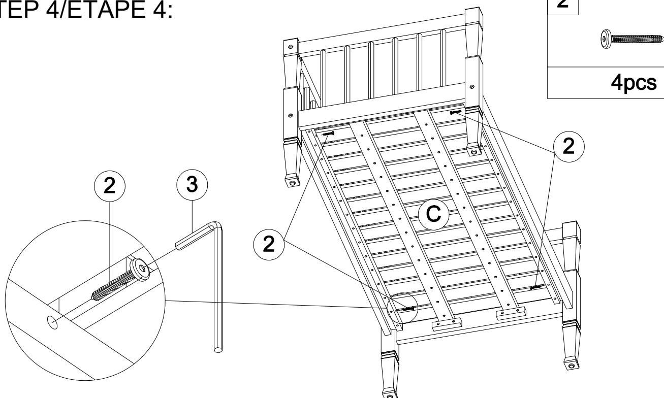
Attach the Seat Panel (C) to the Back Panel (D) & Support bar (E) using Screw (2) and Allen key (3).
