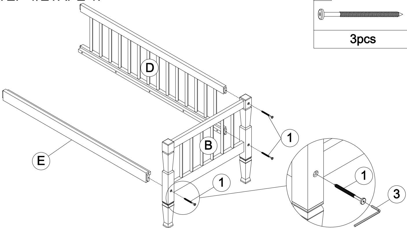
Attach the Back Panel (D) & Support bar (E) to the Right Arm Panel (B) using Screw (1) & Allen key (3).
