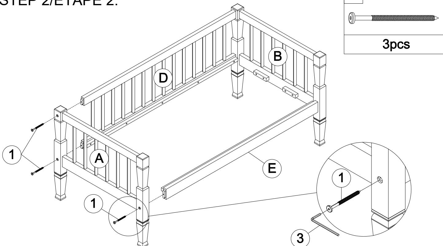
Attach the Left Arm Panel (A) to the Back Panel (D) & Support bar (E) using Screw (1) & Allen key (3).
