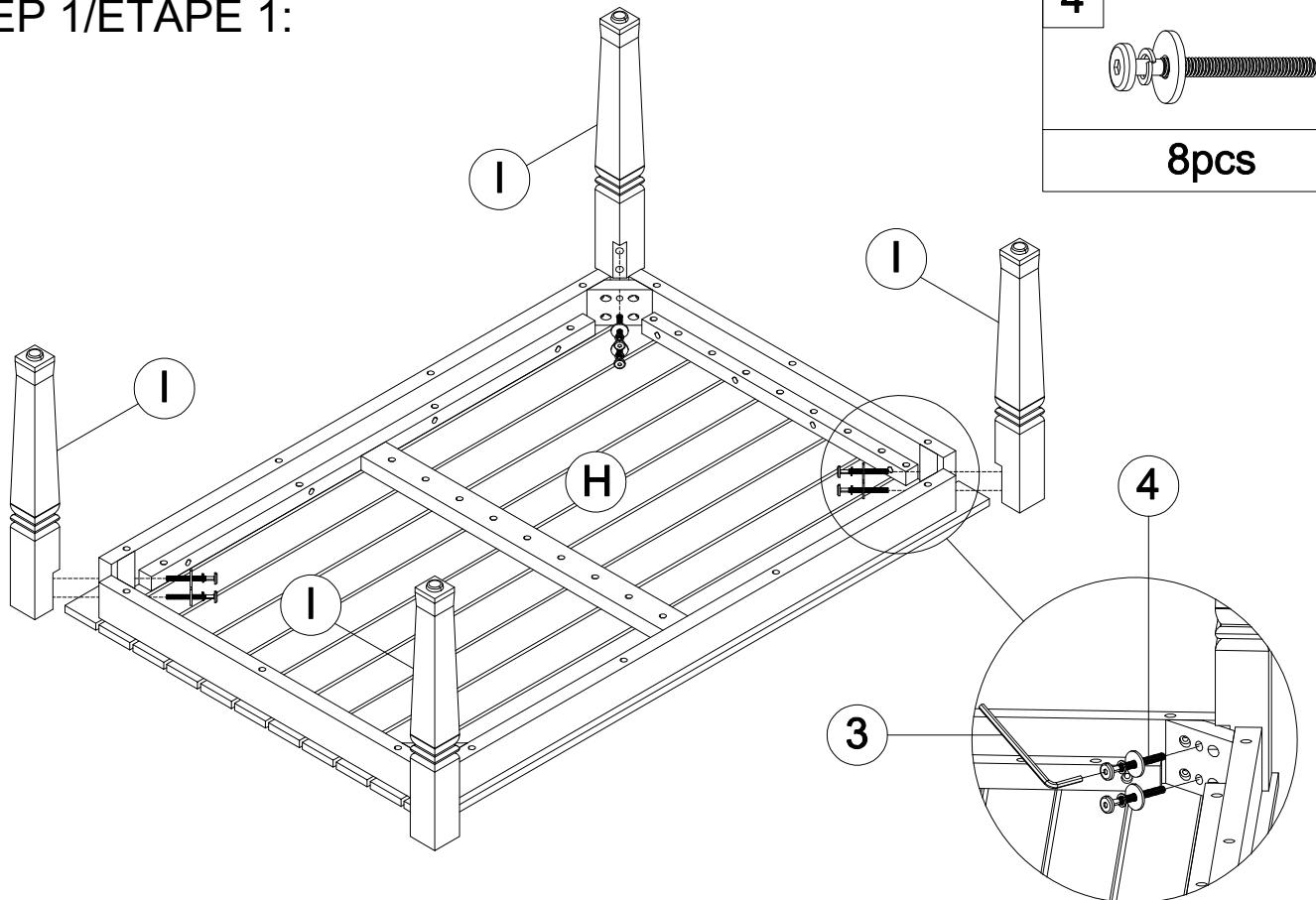
Attach the Legs (I) to the Table Top (H) using Bolts (4) & Allen key (3). Tighten fully all the Bolts./
