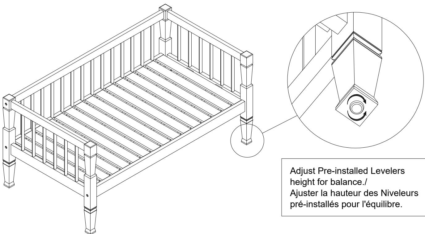
Adjust Pre-installed Levelers height for balance./
