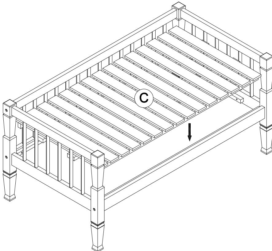
Position the Seat Panel (C) to the Back Panel (D) & Support bar (E)./
