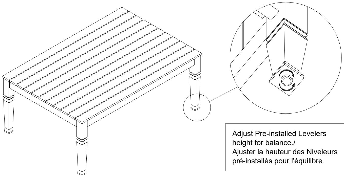
Adjust Pre-installed Levelers height for balance./
