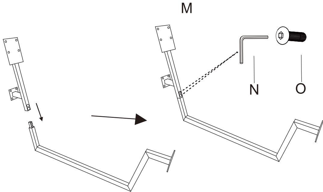
Connect two metal brackets with screws
