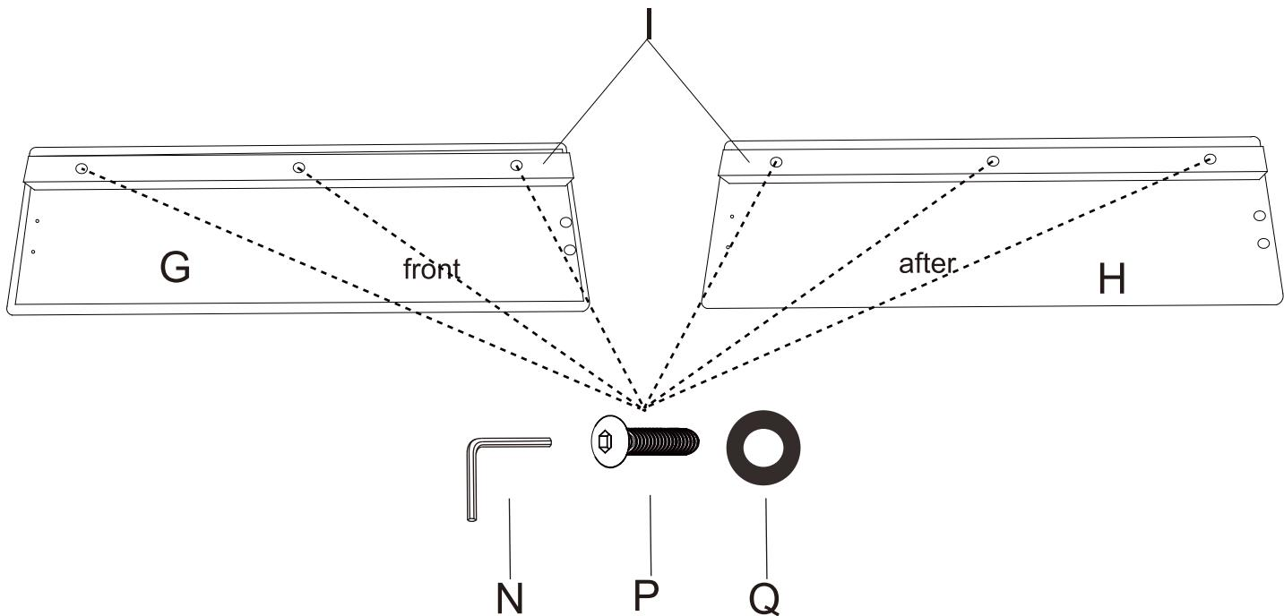
Install the crosspieces(I) onto the front and rear panels(G,H)
