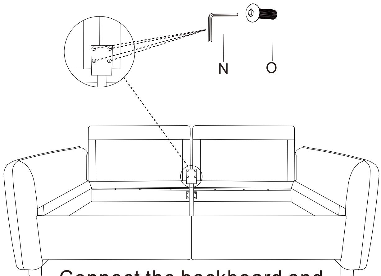
Connect the backboard and metal bracket with screws
