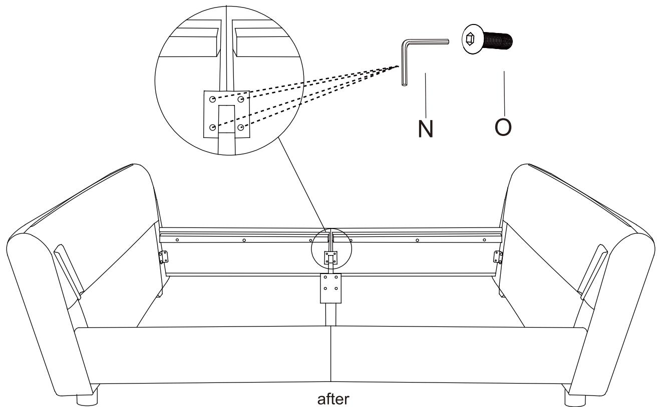
Connect two metal brackets with screws
