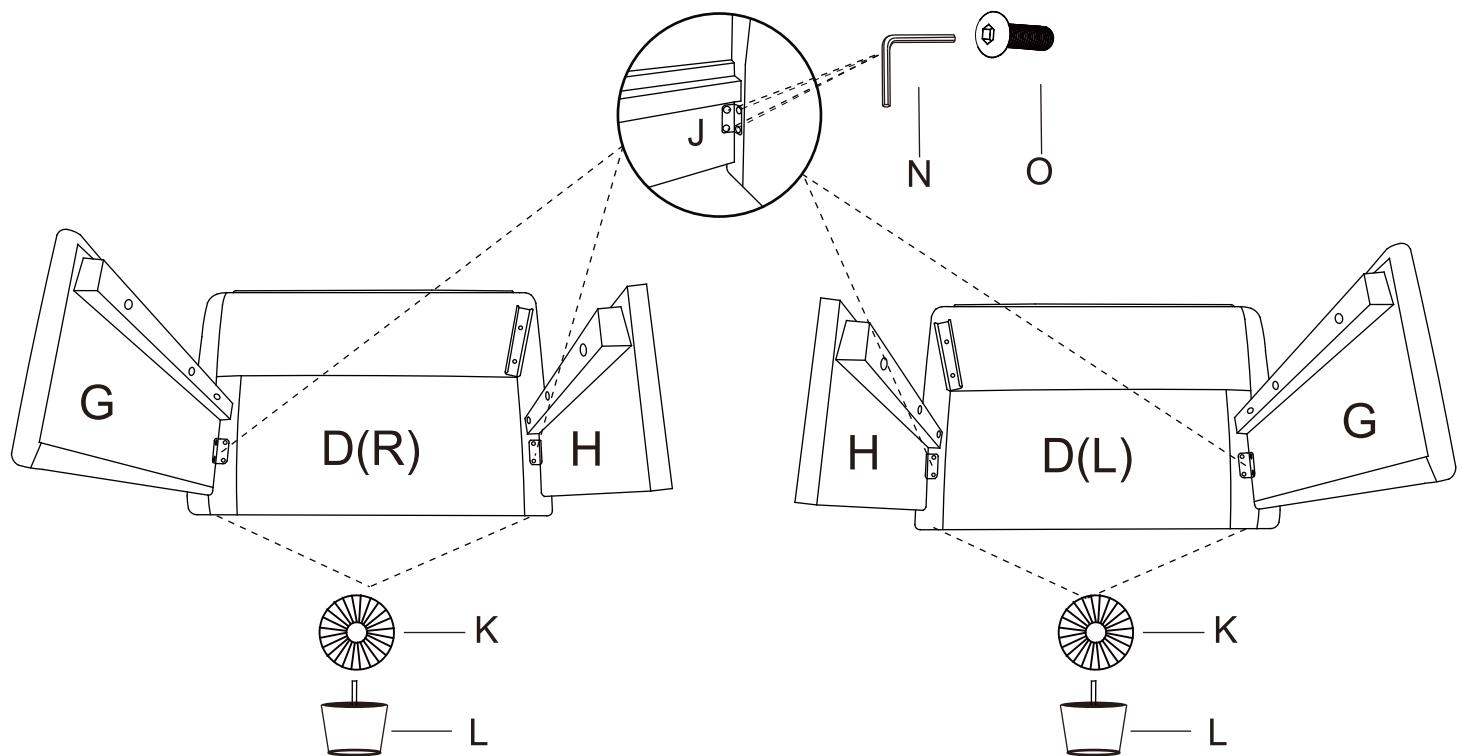
Connect the front and rear panels to the armrest using connectors, and install the plastic feet under the armrest
