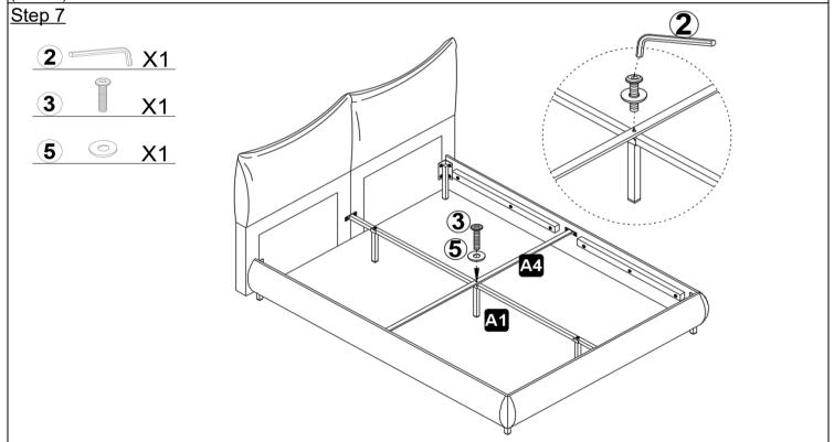
Use Allen wrench (2) screw (3) and gasket (5) to secure the connecting rod (A4) in the bed to the foot in the bed (A1)
