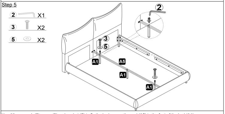
Use Allen wrench (2) screw (3) and gasket (5) to fix the bed connecting rod (A5) to the foot of the bed (A1)
