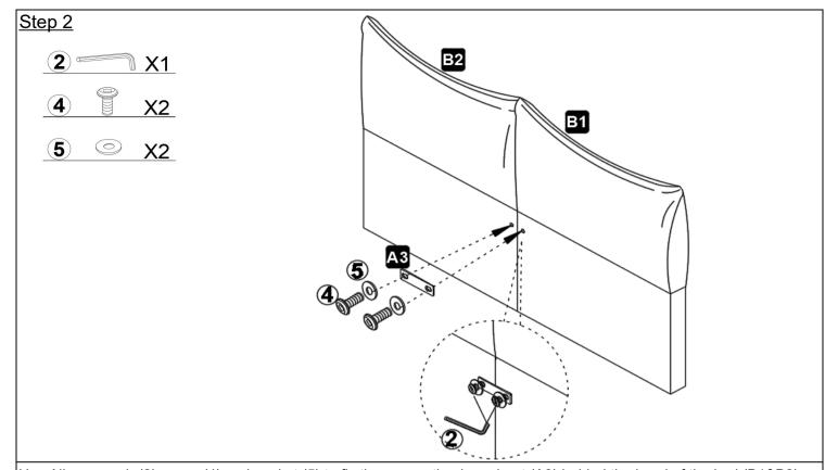
Use Allen wrench (2) screw (4) and gasket (5) to fix the connecting iron sheet (A3) behind the head of the bed (B1&B2).
