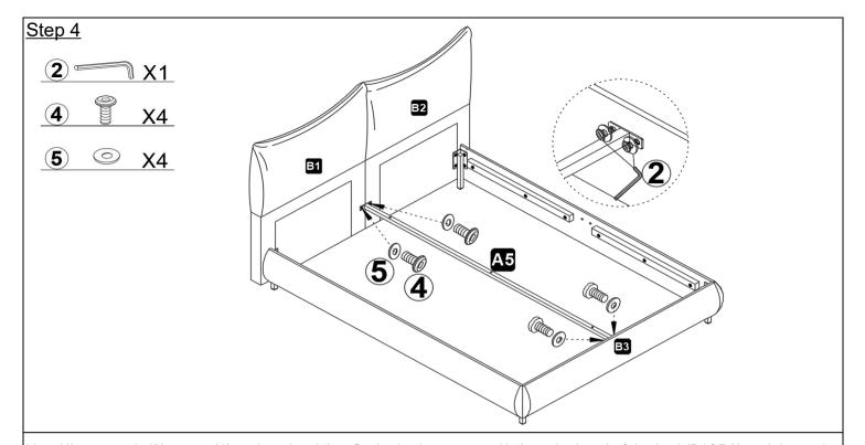
Use Allen wrench (2) screw (4) and gasket (5) to fix the bed connector (A5) on the head of the bed (B1&B2) and the end of the bed (B3)
