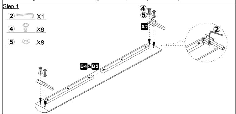
Use the Allen wrench (2), screw (4) and gasket (5) to secure the angle iron (A2) to the bed side plate (B4&B5).
