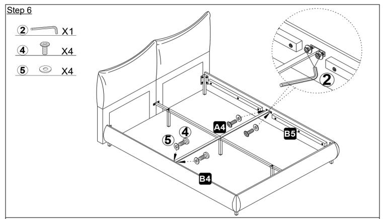
Use the Allen wrench (2) screw (4) and shim (5) to secure the connecting rod (A4) in the bed to the bed side plate (B4&B5).
