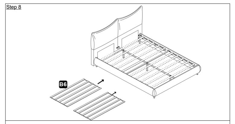
Place the bed frame strip (B6) on the assembled bed frame and paste the magic strip into place.
