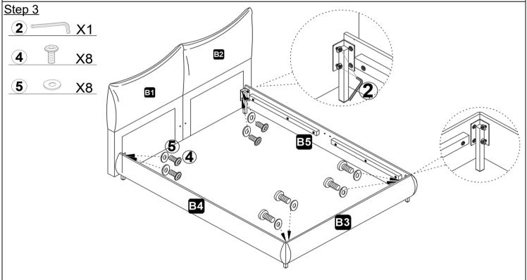
Use the Allen wrench (2), screw (4) and shim (5) to secure the bedside plate (B4&B5) to the bottom board at the head of the bed (B1&B2) and the end of the bed (B3).
