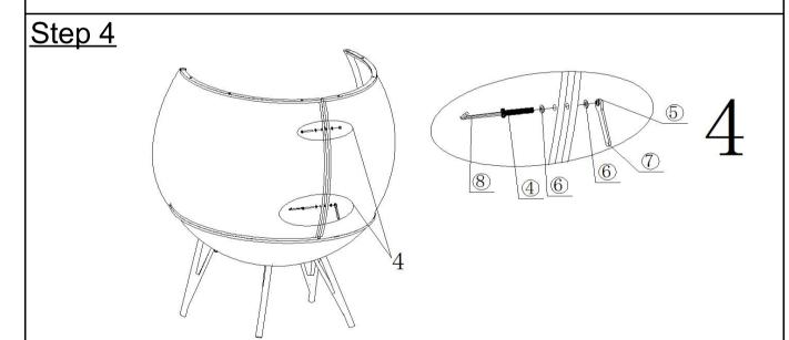
Attach the Middle Right Side Panel(G) to the Middle Left Side Panel(F) with the Allen Key(8) and Wrench (7), using Bolts (4), Washers(6) and Nuts (5).
