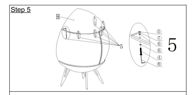
Attach the Basket Top(H) to the Middle Right Side Panel(G) and Middle Left Side Panel(F) with the Allen Key(③) and Wrench (⑦), using Bolts (④), Washers(⑥) and Nuts (⑤). Do not fully tighten the bolts.
