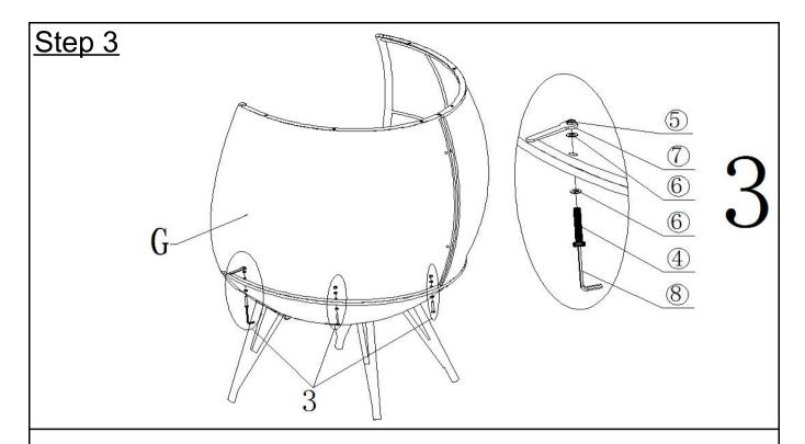
Attach the Middle Right Side Panel(G) to the Basket Seat(E) with the Allen Key(8) and Wrench (7), using Bolts (4), Washers(6) and Nuts (5) .
