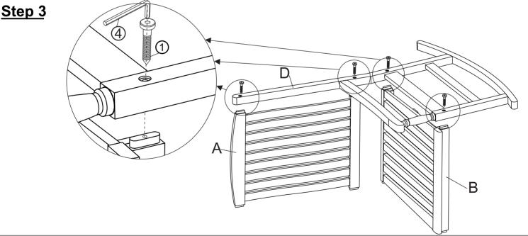
With assistance from your adult partners, put the tenon of Backrest Panel(A) and Seat Panel(B) into the mortise of Right Leg Panel(D) and attach using Screws (1) with Allen Wrench (4).
