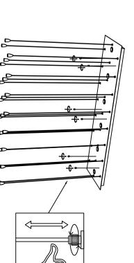
(3) Attach the main lamp frame to the mounting bracket.
