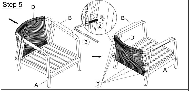
Position the Back Panel (D) to the Left Leg Panel (A) and Right Leg Panel (B) as shown in the above picture.
