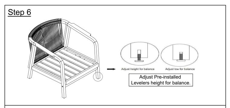
With the assistance from your adult partner, stand the Chair up Inspect the Chair and make sure all parts are adequately connected. Carefully sit onto the Chair. This pressure will help align all parts at all joints.
