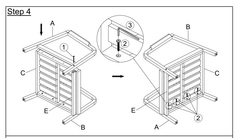
Position the Left Leg Panel (A) to the assembled parts in step 3 and attach to the Support bar (E) using Screw (1) and Allen Wrench (3). After that turn the Chair into the opposite side as shown in the above picture. Attach the Seat Panel (C) to the Left Leg Panel (A) using Bolt (2) and Allen Wrench (3).
