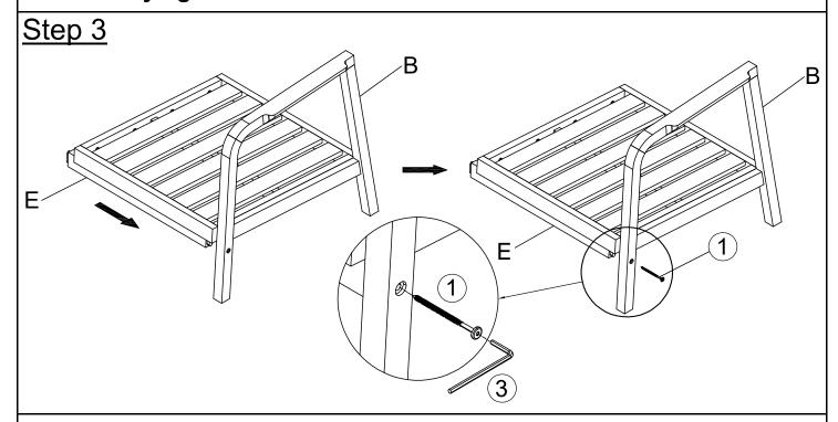
Position the Support bar (E) to the Right Leg Panel (B) as shown in the above picture.
