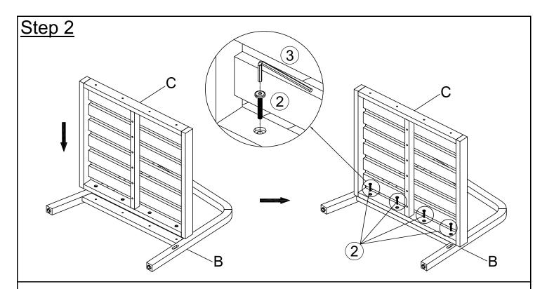
Position the Seat Panel (C) to the Right Leg Panel (B) as shown in the above picture.
