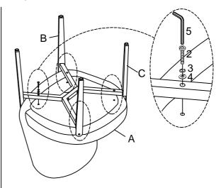
Note: Do not fully tighten the bolts at this step.
