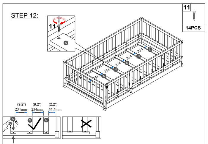
**NOTE:** Please make sure the bed slats close to the side rail before locking the screws to avoid breakage. This step is required for both the left and right sides. Moreover, please do not lock the screws of the bed slats at the outermost edge to avoid damaging.
