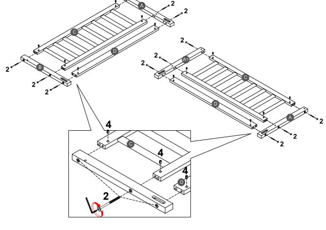
Note:Part 4 will face up with the "x" mark on it, otherwise it cannot be tightened
