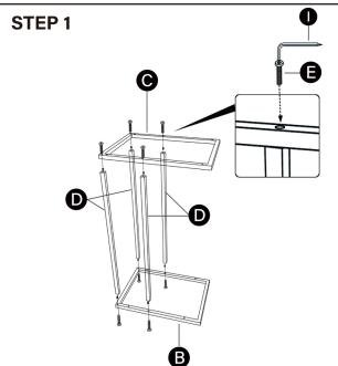
Attach the top frame B and bottom frame C with table legs D using M6x35mm screws.
