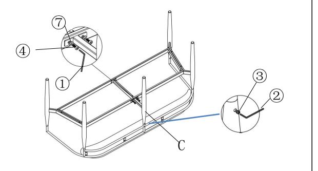
Using Bolts(4) and Washer(7) with Allen Wrench(1) and Bolts(3) with Allen Wrench(2) to connect the Middle Hind Leg (C) to the Legs Connection (E) and Backrest (F) as shown above. **DO NOT FULLY TIGHTEN THE BOLTS.**
