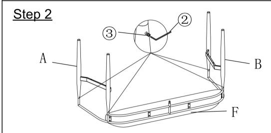
Attach Left Leg (A) and Right Leg(B) to the Backrest (F) using Bolts(③) with Allen Wrench(②). **DO NOT FULLY TIGHTEN THE BOLTS.**
