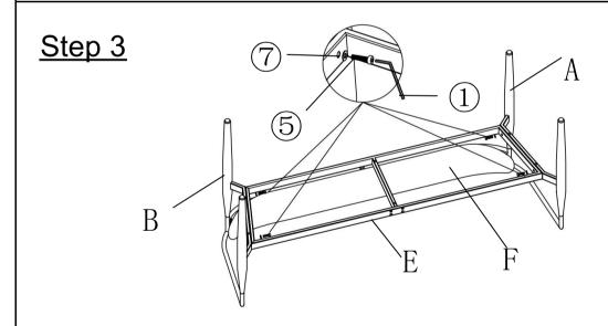
Attach Legs Connection (E) to the Left Leg (A) and Right Leg(B) using Bolts ( $\mathfrak{G}$ ) and Washer ( $\mathfrak{T}$ ) with Allen Wrench( $\mathfrak{T}$ ) as shown above..
