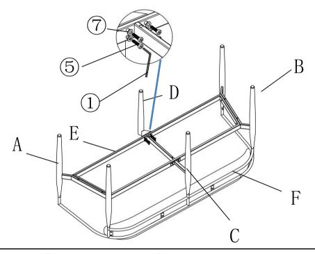
Using Bolts(5) and Washer(7) with Allen Wrench(1) to connect the Middle Front Leg (D) to the Legs Connection (E) as shown above.
