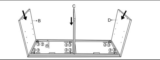
Attach the right side boad(B), left side board(D) and middle clapboad (C) to the top panel(A), use long bolt(②) and flat washer(③) align with board hole position, Allen wrench (④) is used to assist rotation tightening. ATTENTION: All the grooves must be stay in one side(backside). The short distance from the edge to the hole is upside for middle clapboard(C).
