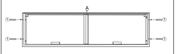
Install the Wooden Tenons(1) into the sides of the Top Panel (A) as picture above.
