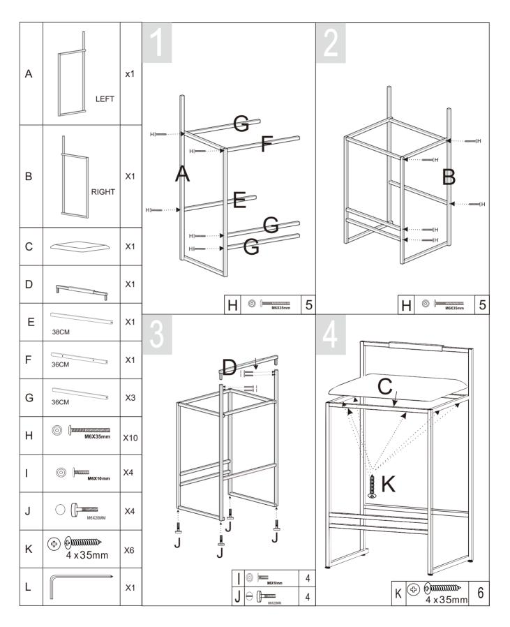
NOTE: There are no screw holes in seat C, seat C is made by wooden frame, please pass through the holes in metal frame with self-tapping screws (part K), then secure seat C by tightening self-tapping screws (part K).
