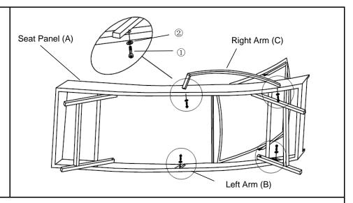
Open the back, Attach Right Arm and Left Arm to the Seat Panel using Bolts (1), and Washers (2), with Allen Key (3).
