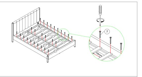
Attach all Slats (F), (F1) to the rail on Side Panel (G), (H) by using Screws (⑦) and Screwdriver (Not Provided).
