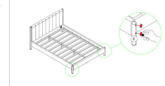
Apply Sticker (9) to cover the bolt holes on the Footboard Leg (E).
