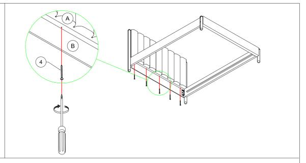
Using Screws (4) and a Screwdriver (Not Provided) to secure the Headboard (B) to the Headboard (A) from below at the pre-drilled hole positions. Be sure to turn the Screwdriver straight
