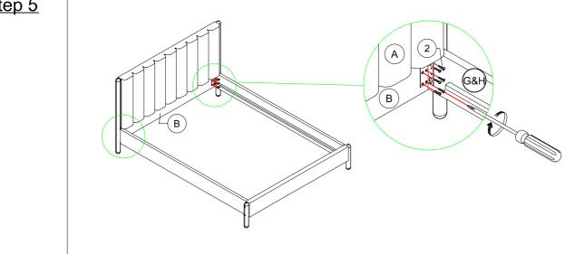
With the help of your partner, keep the Headboard (B) parallel to the Headboard (A). Then, secure it to the steel bracket (1) by using Screws (2) and a Screwdriver (Not Provided).
