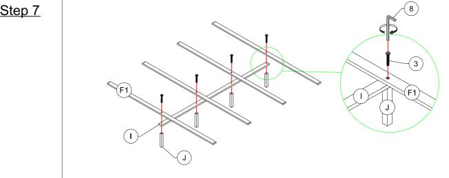
Align the Mounting Position on the Center Rail (I) to the Center Leg (J) and the Slat (F1). Attach the Slat (F1) and the Center Rail (I) to the Center Leg(J) and by using Bolts (③), with Allen Wrench (8).
