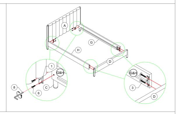
With the help of your partner, stand the completed Headboard from Step 2 and the Footboard (D) from Step 3 upright as shown in the picture above. Affix the Side Panels (G) and (H) to the Headboard Leg (C) and Footboard (D) using Steel Bracket (1) Bolts (3), Bolts (6) with Allen Wrench (8).
