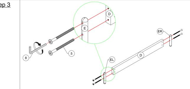
Align the Mounting Position of Footboard Leg (E) into the Mounting Position of Footboard (D) as shown above. Affix the Footboard Leg (E) to Footboard (D) by using using Bolts (5) with Allen Wrench (8).
