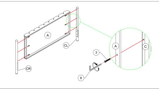
Align the Mounting Position of Headboard Leg (C) into the Mounting Position of Headboard (A) as shown above. Affix the Headboard Leg (C) to Headboard (A) by using using Bolts (③) with Allen Wrench (®).
